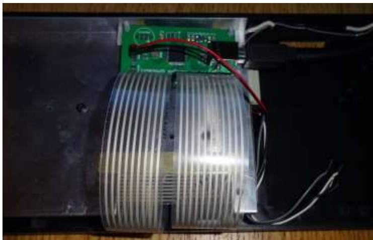
The keyboard membrane plugged into the USB controller board mounted on the QL keyboard back=plate
